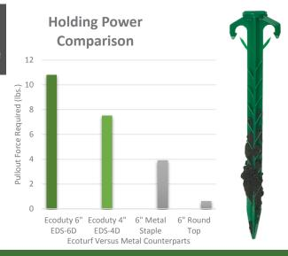
3rd Party Testing was conducted by Trace Laboratories, Inc. located in Palatine, IL 60067.
