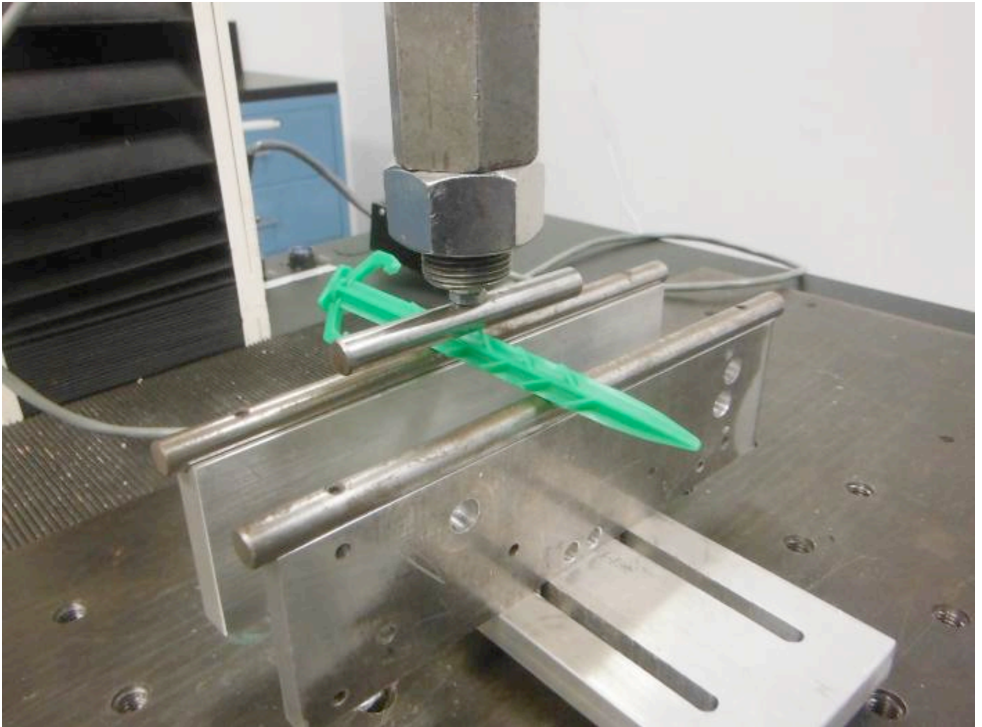
Bend Test Setup
